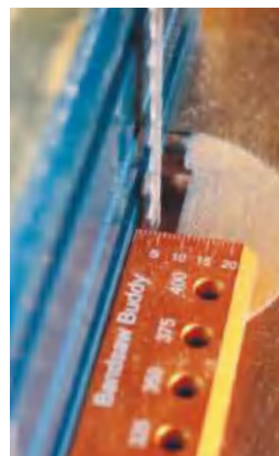
▲ This simple ruler scale makes it easy to set up veneer rips
